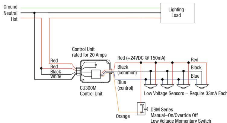
DSL Series with CU300A, Override Off Single Circuit:
