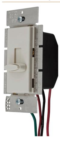
Hubbell tradeSELECT® preset slide dimmers provide the precise control of full range dimming with an on/off button feature built into the slide. Press on, adjust the slide to change the light level, press off. Featuring an additional 3-way wire lead, this dimmer can be used as either a single pole or 3-way, thereby reducing the need to stock additional units. Designed to compliment the decorator look, they are available in white, ivory and light almond.
